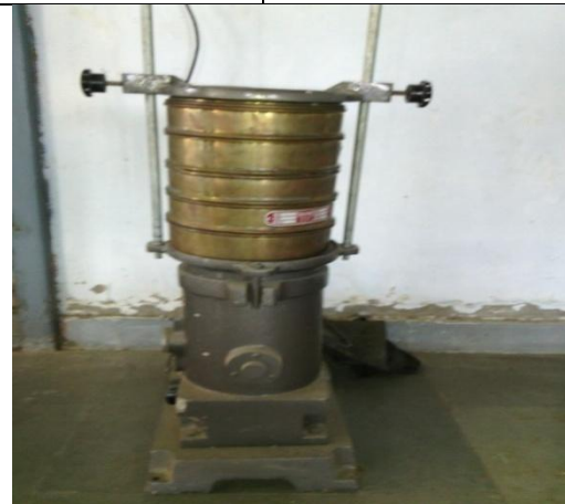
Fig. 1: Photograph of vibrating sieve setup
