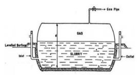
Fig -3: Flexible Bag Type Digester
