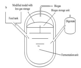
Fig -2:Schematic Diagram of Fixed Dome Digester
