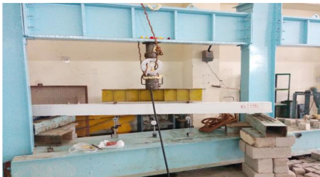
Fig -3: Test setup of a beam subjected to Loading
