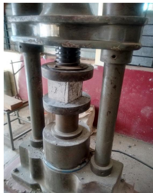
Fig-1: Compression strength test setup.
