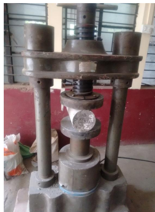
Fig-1: Compression strength test setup.
