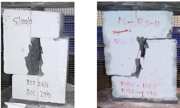
Fig -9: Failure pattern in end-block strengthened self-compacting concrete push-off specimens
