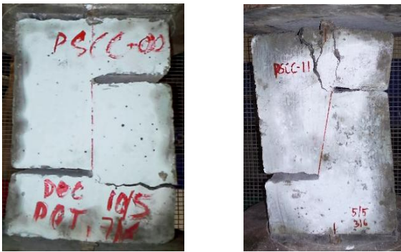
Fig -8: Failure pattern in plain self-compacting concrete push-off specimens
