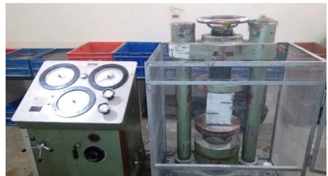
Fig -6: Compression testing machine used for testing
