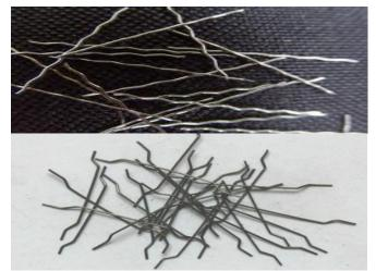
Fig -1: crimped and hooked steel fibres
