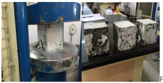
g -3Cube specimen under test Table-3: Compressive strength Results
