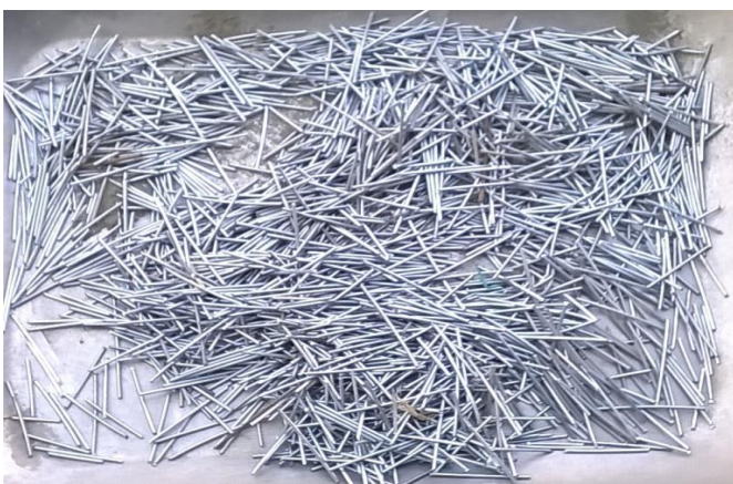
Fig. 2 Samples of Galvanized steel fibres
