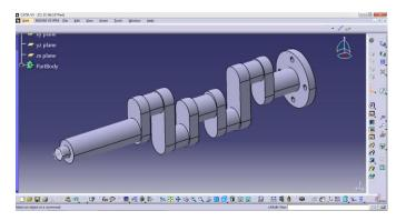
Fig -1: 3-D Model of crankshaft using CATIA V5
