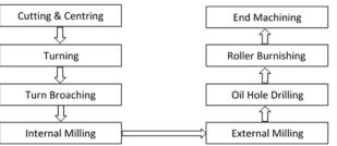
Chart -4: Machining process for manufacturing crankshaft
