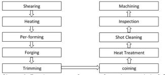
Chart -2: Forging process for manufacturing crankshaft [2]
