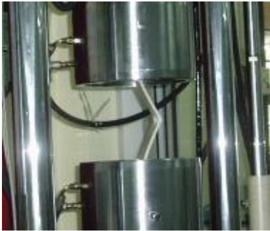
Fig 4 Compression of specimen
