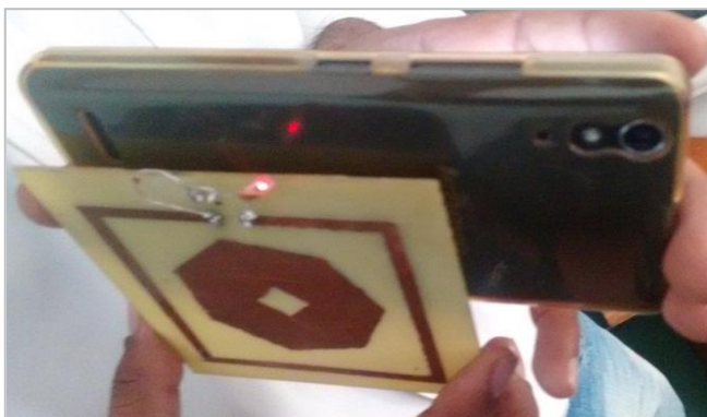
Fig- 10: Experimental demonstration of proposed system by LED glowing.
