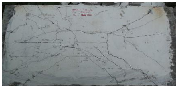
Fig -3.1: Typical crack pattern of TVC slab (tension side)
