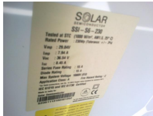
Fig.2: Details of Solar panels
