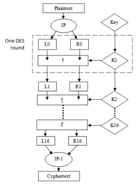
Fig 1.2 DES Core Algorithm
