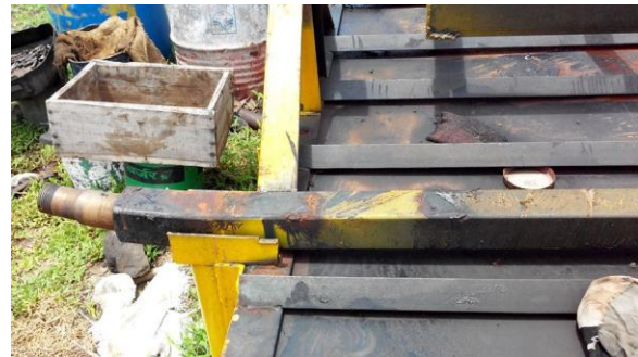
Fig2. bending problem of square axel trolley
