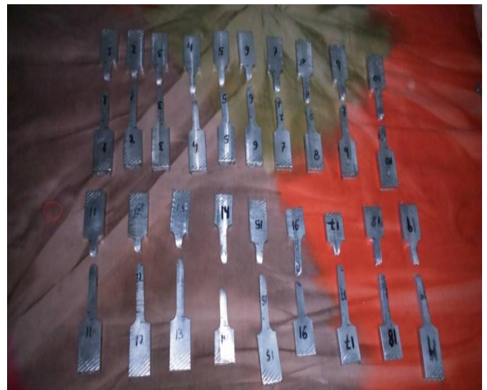
Fig.3.2-Specimens after tensile testing
