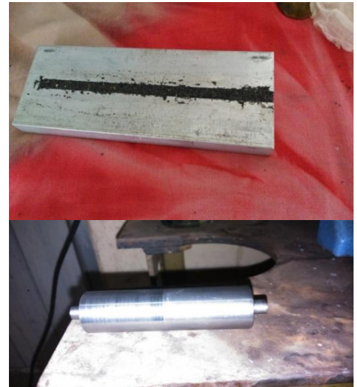
Fig.2.1-Sic reinforced in the groove of the base metal and plain cylindrical tool used for FSP
