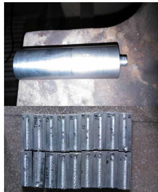
Fig.2.2-Threaded cylindrical tool and Set of FSP specimens
