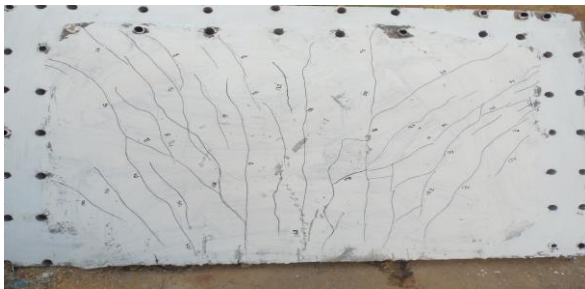
Fig -8: Crack pattern of HSTVC slab with 0.25% fiber @ tension face.
