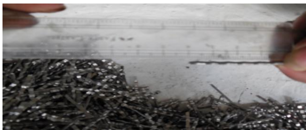
Fig -2: Crimped steel fibers
