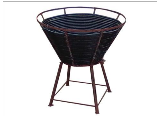
Fig 2: 3-D Representation of Conical frame with spiral tubing
