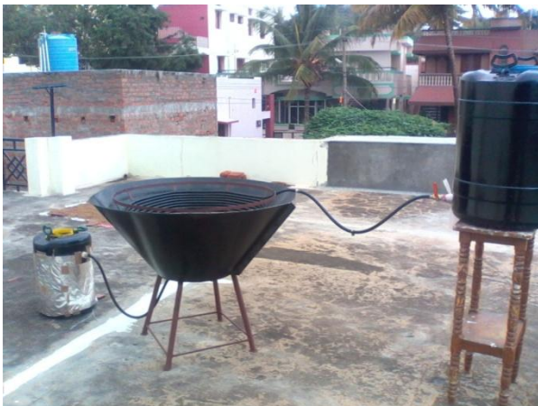
Fig 4: Actual experimental setup of solar water heater
