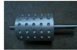
Fig-4: Cavitation heater rotor side view after machining.
