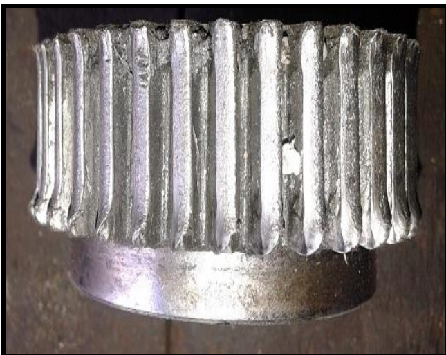
Fig -2: View of spur gear with wear
