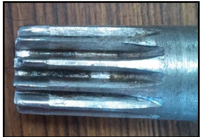
Fig -4: View of pinion with tooth breakage
