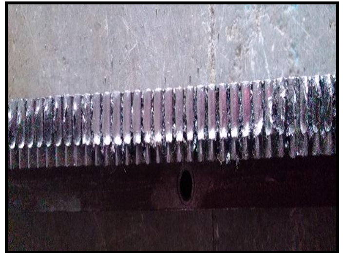
Fig -3: View of rack with wear failure
