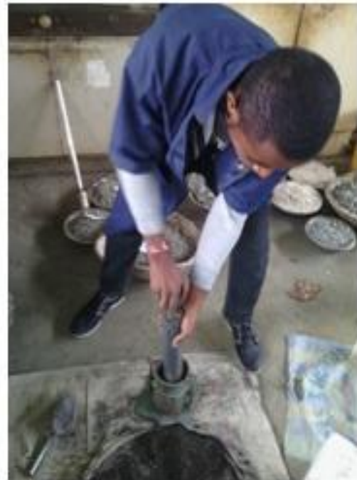
Fig. 7: Picture showing compaction Test
