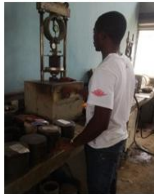
Fig. 8: Picture showing Unconfined compression test
