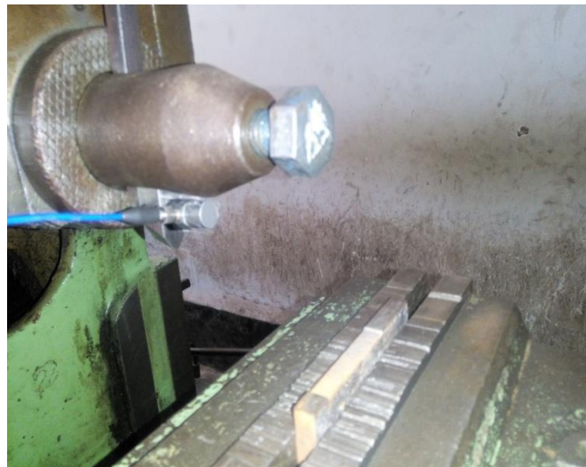
Fig -2: Accelerometer mounted on the tool during working of machining
