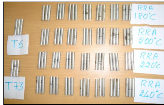
Fig. 1 Photograph showing real test specimen utilized for wear test
