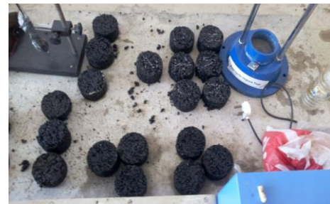
Figure 4 Blends of Aggregate and Bitumen and blends of Aggregate-bitumen-plastic mix
