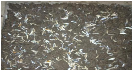
Fig- 2 Bottle cap fibers added to concrete
