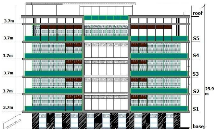
Fig 2: Elevation View of Building
