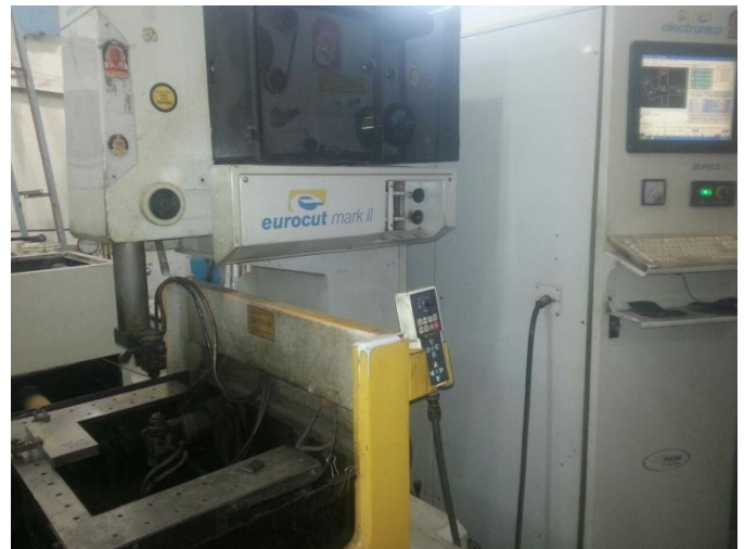
Fig.-2: Workpiece mounted on EURO CUT MARK II machine
