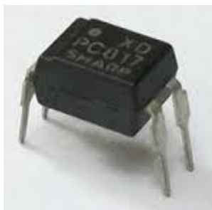
Fig -4: Optocoupler PC817
