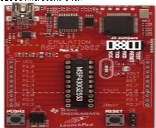
Fig -2: MSP430G2553 Microcontroller
