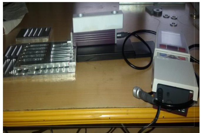
Fig.2. Set up for surface roughness measurement
