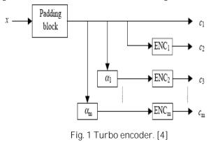
The input of the TC encoder is a data block x, with k information bits. To this information sequence the padding block appends v (memory size) tail bits, which then yield the
