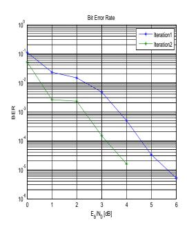
Fig 6 BER plot for log-map decoder: Unpunctured [4]
