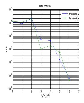
Fig 7 BER plot for SOVA decoder: Punctured
