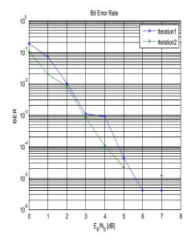
Fig 8 BER plot for SOVA decoder: Unpunctured [5]
