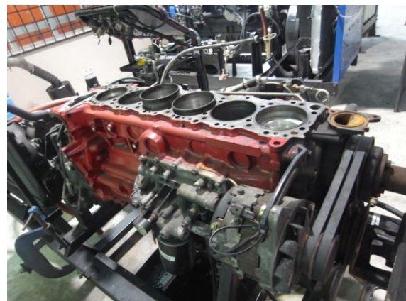
Fig - 1: The First Prototype of CNG Conversion Engine (HINO, J08-T1 Model with 6 Cylinders and Displacement of 6,691L Diesel Engine)
