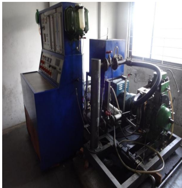
Fig: 2 shows EGR set to the Single cylinder Diesel Engine
