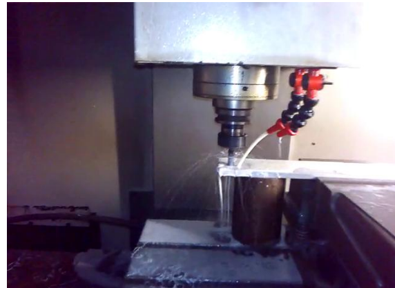
CNC milling operation using VML-800.
