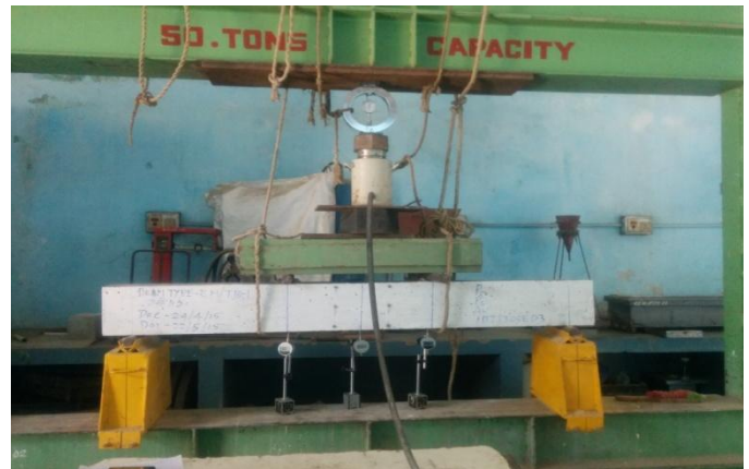
FIG 5: Test set up on loading frame
