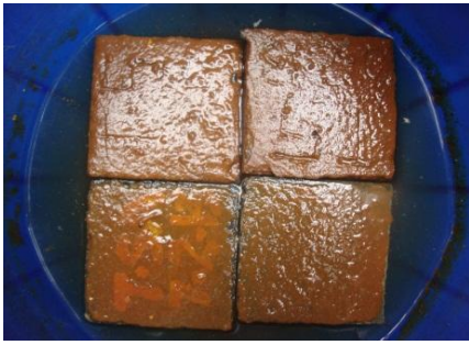
Fig. 4 Cubes under Acid Attack
