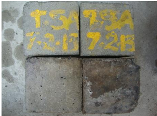
Fig 5 Cubes under Alkaline Attack
