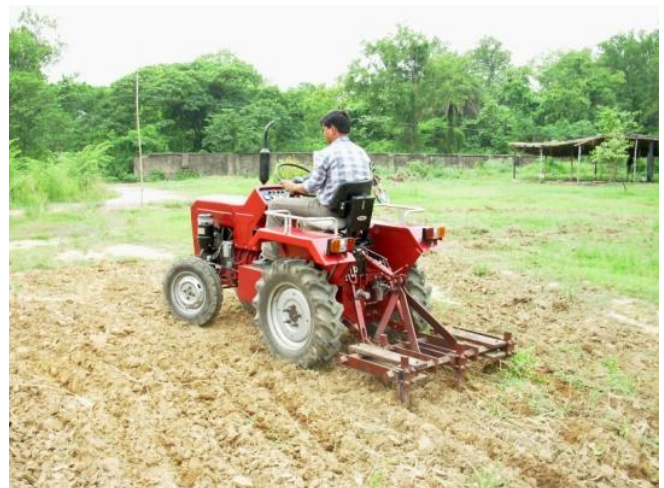
Fig.5: Field trial of the cultivator with a Low HP Tractor
