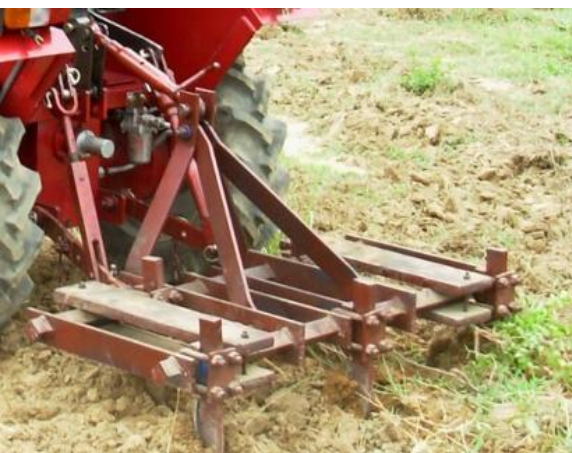
Fig.3: Physical prototype of the developed cultivator attached with a Low HP Tractor
