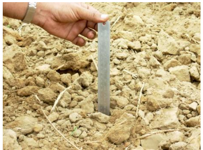
Fig.6: Depth of cut measurement during field trial of the cultivator
