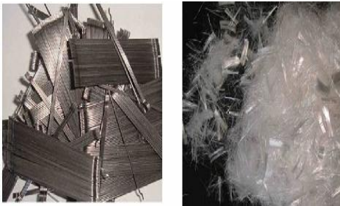
Fig- 1: Steel Fiber with Hooked-end and Polypropylene Fiber
