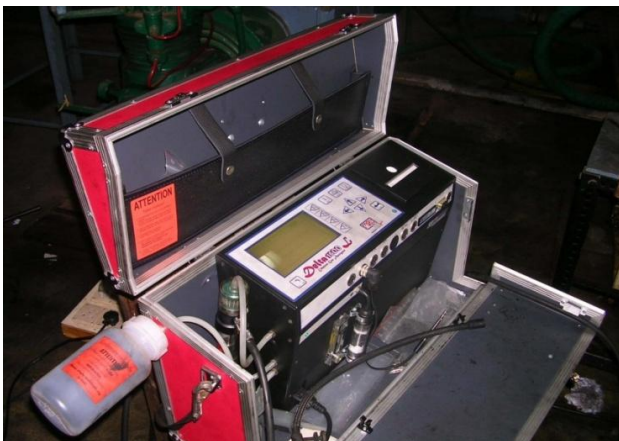
Fig -4: Exhaust Gas Analyzer
