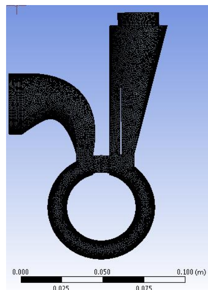
Fig 5: 3D Mesh of fluid region
