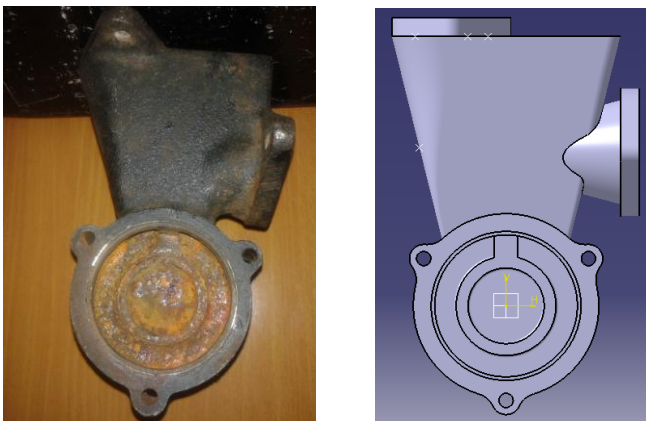
Fig 2: Image of Actual Pump Casing and its CATIA Model
