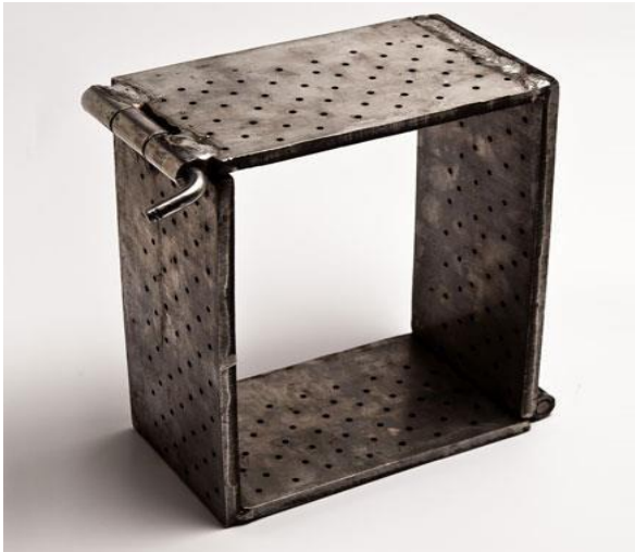
Fig-5: Mold Box
