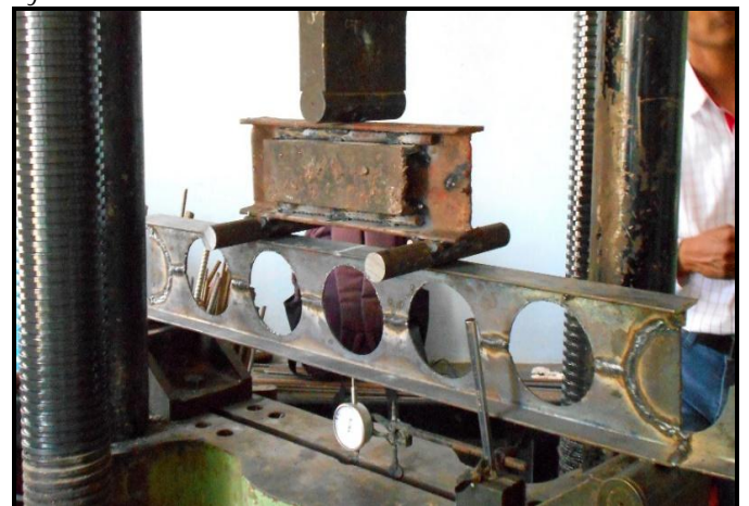
Fig -12: Test set up of circular castellated beam
