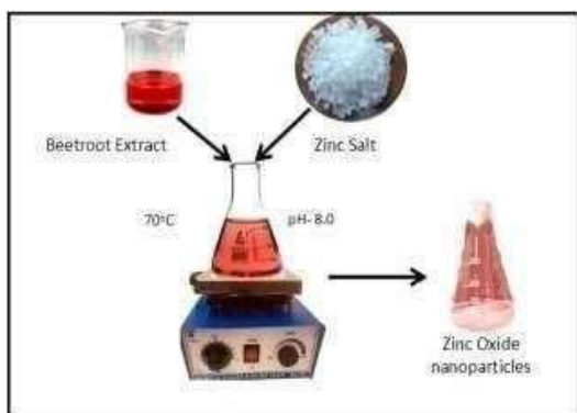
Figure 2. Schematic Representation of formation of Zinc-oxide Nano-particles
