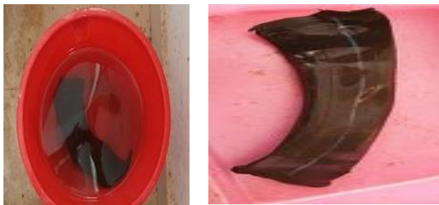
Fig: Water absorption test on rubber
