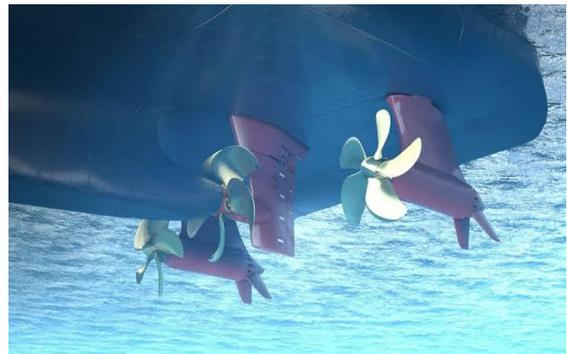
**Figure 3. 2 or more propeller in the aft of the ship to create additional waves**
