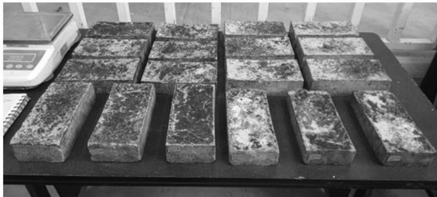
Fig. 1. View of samples obtained from various PET-basalt mixtures with dimensions of 200 x 100 x 60 mm.
