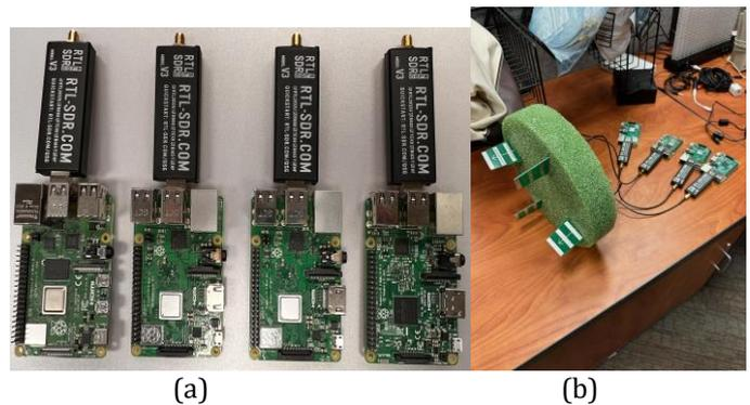
**Fig-4.** (a) Initial hardware configuration. (b) Directional antennas mounted in a Styrofoam disc.
