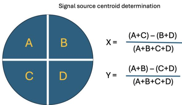
**Fig-2.** Optical quadrant detection centroid determination.
