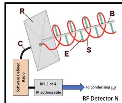
**Fig-1.** Directional antenna, software defined radio (SDR) and microprocessor are the principal components of the radio detection portion of the device.
