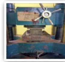
Fig-4: Compressive strength test in UTM
