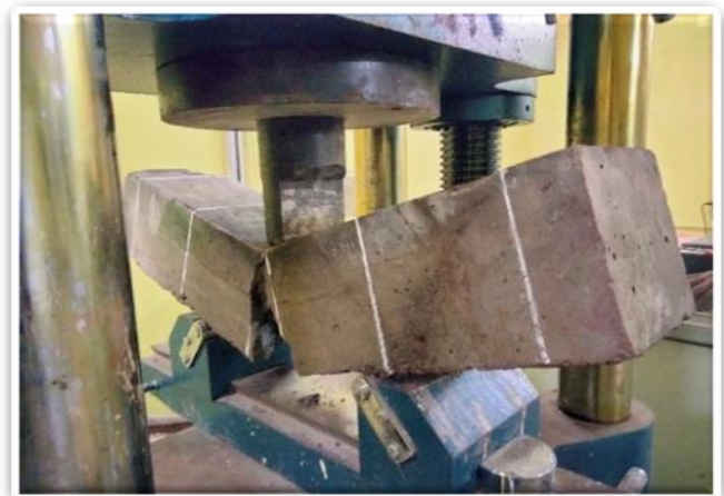
Fig-6: flexural strength test of concrete in UTM
