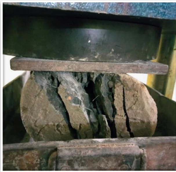
Fig- 5: Split tensile strength test in UTM
