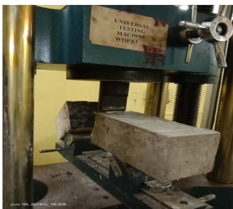
Fig- 4: Flexural strength test in UTM
