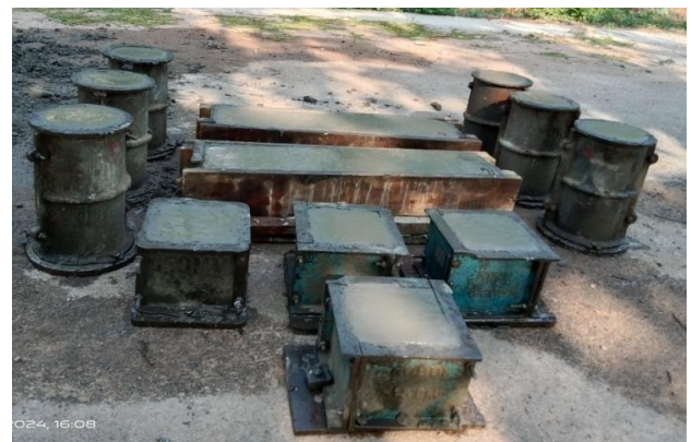
Fig-1: Casting of Cube, Beam and Cylinder.
