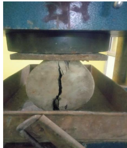
Fig- 3: Split tensile strength test in UTM
