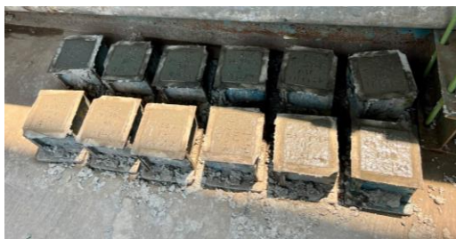
Fig -2: Concrete cube for testing
