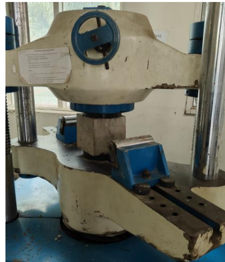
Fig-7: Compression testing of cubes
