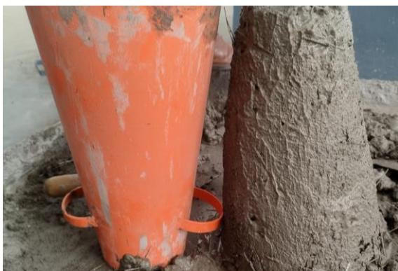
Fig-10: Slump Test on freshly prepared concrete
