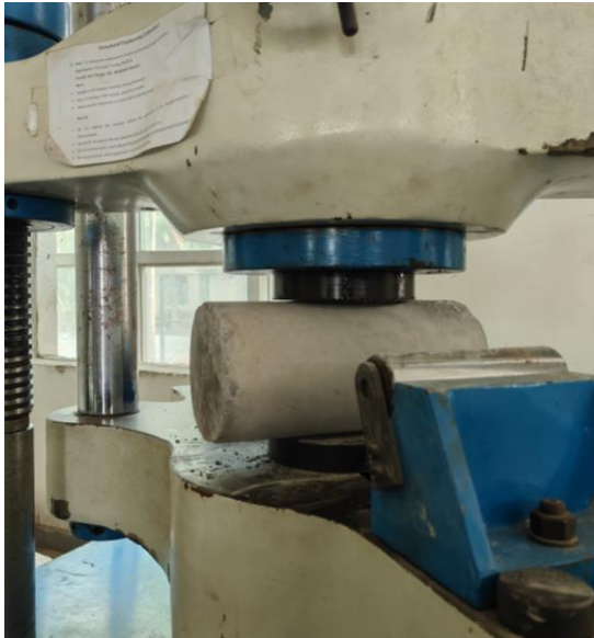
Fig-9: Split Tensile Test of cylinders
