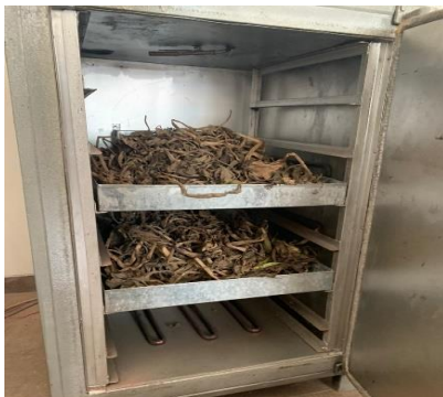
Fig-2: Oven drying of water Hyacinth
