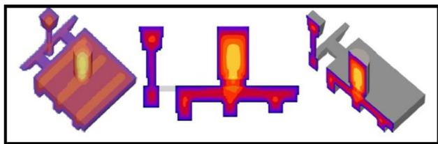
Figure: 2.4 Casting Solidification Simulation
